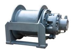
GMW series hydraulic winch is composed with all sorts of distributors that consist of one-way balance valve, control brake, high pressure shuttle valve, GM type hydraulic motor, Z type brake, C type gearbox, and drum. Users only configure hydraulic power unit and change valve. As the winch has valve sets, its not only simplified the hydraulic system, but also enhances the working reliability of the transmission drives.
